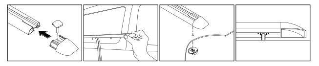
Gently Finger tighten T-bolts only at this stage. Once all have been started then tighten in the pattern as shown below. Ensure all knobs are in line as shown. **DO NOT OVER TIGHTEN.**
