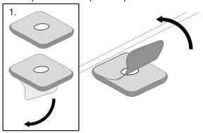
Install track end caps. Remove paper gasket from foam tape on underside of track. Place tracks onto canopy / hard tonneau. Ensure the cut outs are placed toward the rear of the vehicle. Double check that all T-bolts have o-rings fitted.
